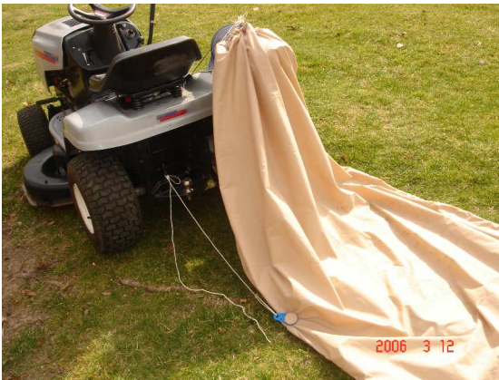
Fig 3- Leaf Bag and Tow Rope attached to the tractor. Note bag clip is on side of bag, in line behind tractor.
