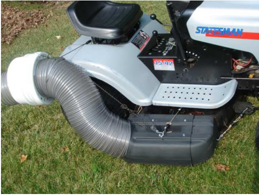
Fig 1- Discharge Tube attached to side of lawn tractor w/ rope ratchet at top, hooked to tractor where convenient.
