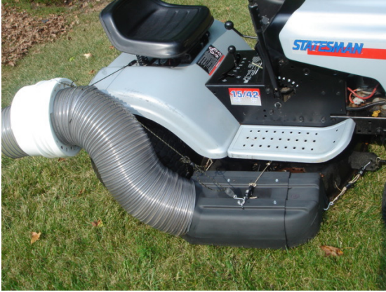
Fig 1- Discharge Tube attached to side of lawn tractor at top, and from DA to Chute Vent Disk.
