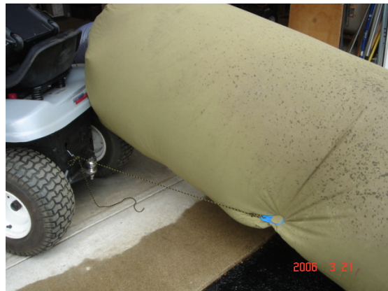
Fig 4- Leaf Bag in use and towrope carrying the weight of the leaf bag.
