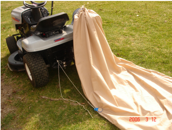
Fig 3- Leaf Bag and towrope attached to the tractor. Note bag clip is on side of bag, in line behind tractor.
