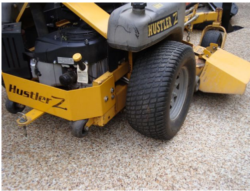
Tire sticks out past the fender/gas tank.
