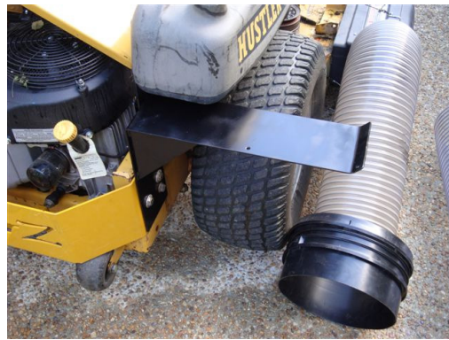
Fancy bracket installed to support discharge tube.
