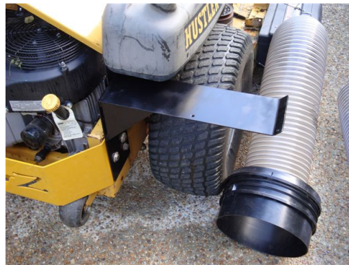
Fancy bracket installed to support discharge tube.
