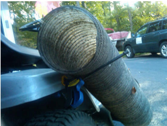
Tube sitting on clamp, secure with cord.
