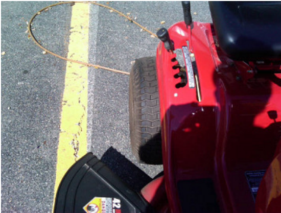
Tire exposed and controls in fender.
