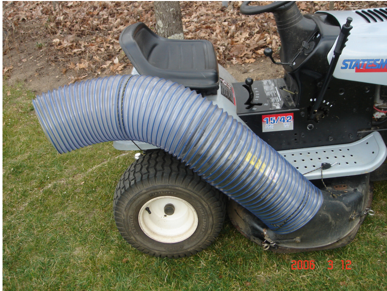
Picture #1- Tube with ratchet hold down at top and hooked to tractor where convenient.
