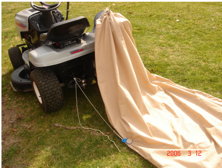
Picture #3- Leaf Bag and Tow Rope attached to the tractor. Note bag clip is on side of bag, behind tractor.
